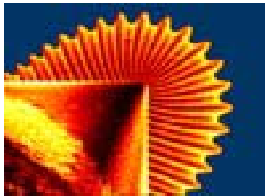
SEM of a Charged Diamond Tip
